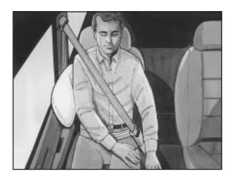
The seat-mounted side impact airbag for the right front passenger is in the side of the passenger's seatback closest to the door.
